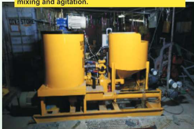
MMA Cement grout Pump 400litre capacity Screw Type pump, electrically operated . Attached with Accelerator Pumping arrangement in same frame& Fitted with VFD, RPM control for mixing and agitation.
