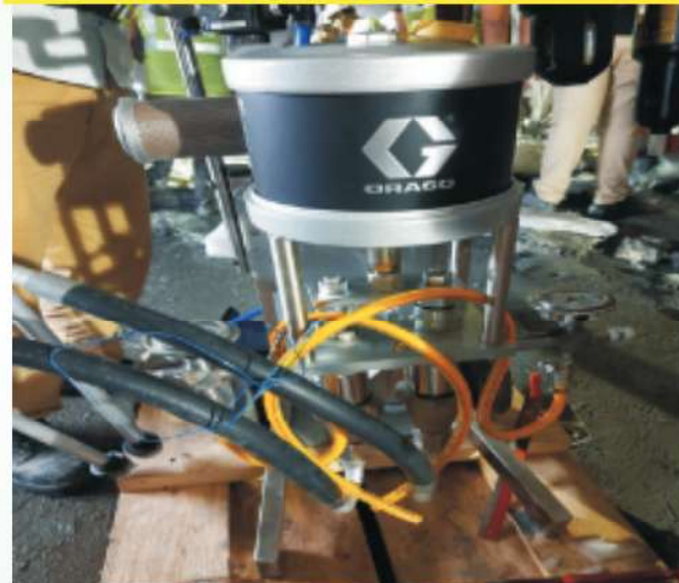
We have Two nos Twin PISTON Chemical Grouting Pump For 2K PU resin and 2K Acrylate Injection Grouting with maximum grouting pressure up to 150Bar.
