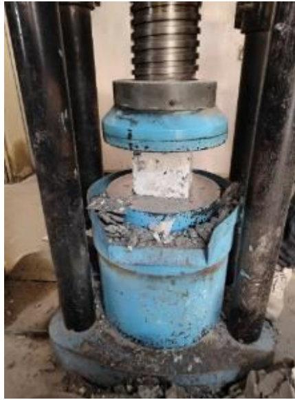
Figure 6. Testing and failure of 150 mm cube specimen.
