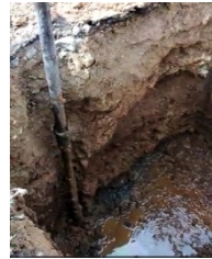
Flow of water observed at BH – 4, d = 2.0m
